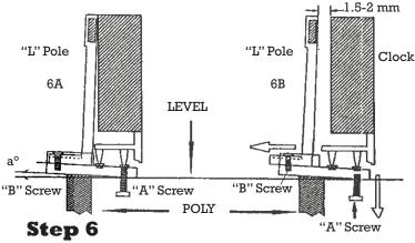
If the pendulum is not level as shown in picture 6A then you may need to move the "L" pole slightly left. This is achieved by screwing down screw "B" to make the pole "L" vertical and the gap to the clock 1.5-2mm. You can also slide the pole "L" back and forth to achieve the correct gap as shown in picture 6B.
